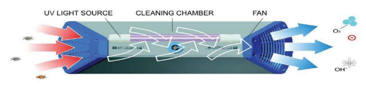
\*Air does not need to pass through the chamber to be purified due to the unit transmitting ozone, photoplasma and negative ions.
